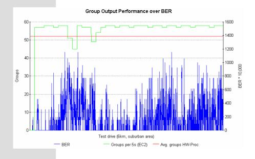
Investigation showing the number of RDS groups, output by the baseband decoder. Originating from a typical mixed-signal reception test drive 1) 2)
