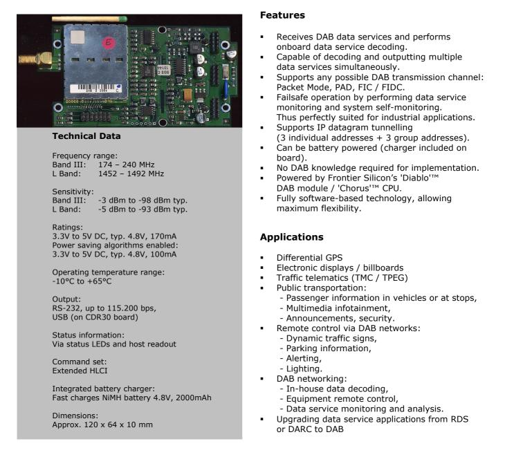
CDR20 is a compact, standalone, highly reliable data receiver board, primarily designed for industrial DAB applications. The receiver performs the entire DAB data service decoding. No further processing of received data is required on the target system. This enables the target system to handle the DAB transmission chain transparently, just like a cable or a modem interconnection.
